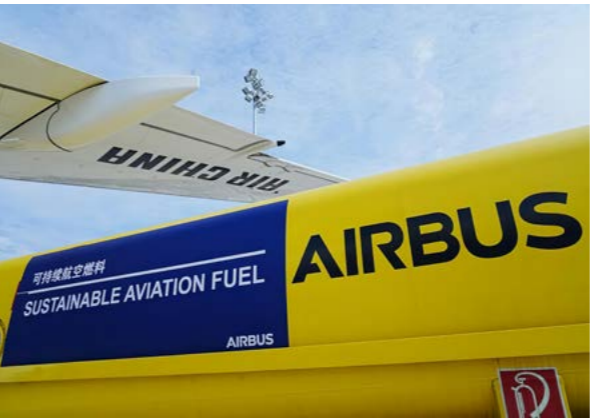
Source: Airbus (China) Enterprises Management and Services Co., Ltd. Figure 2: Airbus Tianjin uses a dedicated SAF tanker for physical segregation
