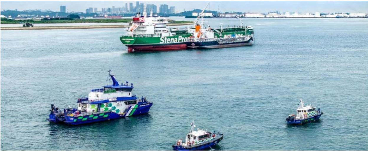
Ship-to-ship bunkering of blended methanol for the Stena Prosperous
